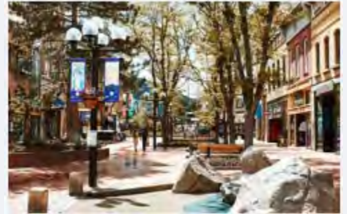
The width of the fire lane for Boulder’s Pearl Street Mall is just 12 feet, within which lie a number of permanent landscaping features.
